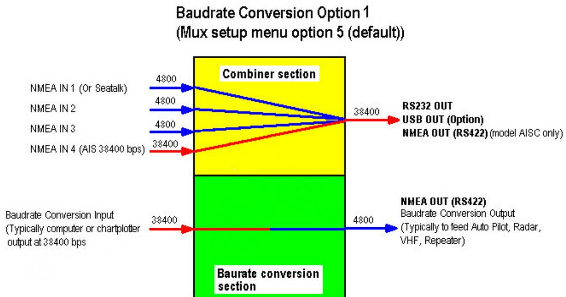
**Combiner and Baudrate conversion work independently. There are no data-paths between the two processes.**
