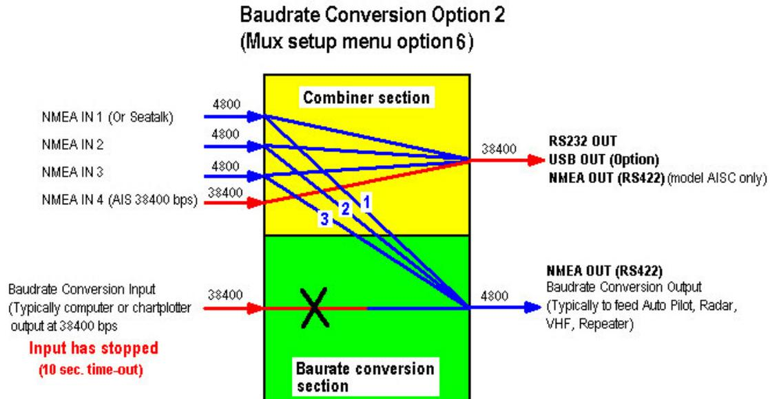
If Baudrate Conversion input is present, the mux behaves the same as for Baudrate Conversion option 1
