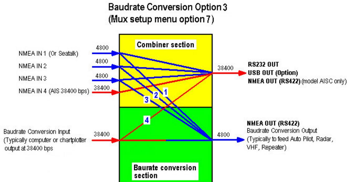
Data from NMEA inputs 1, 2 and 3 is also included in the baudrate conversion output stream.
